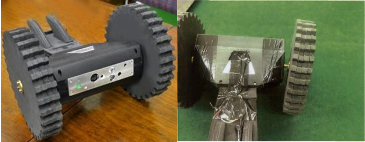
Figure 6 SCARAB robot and bent motor shaft
