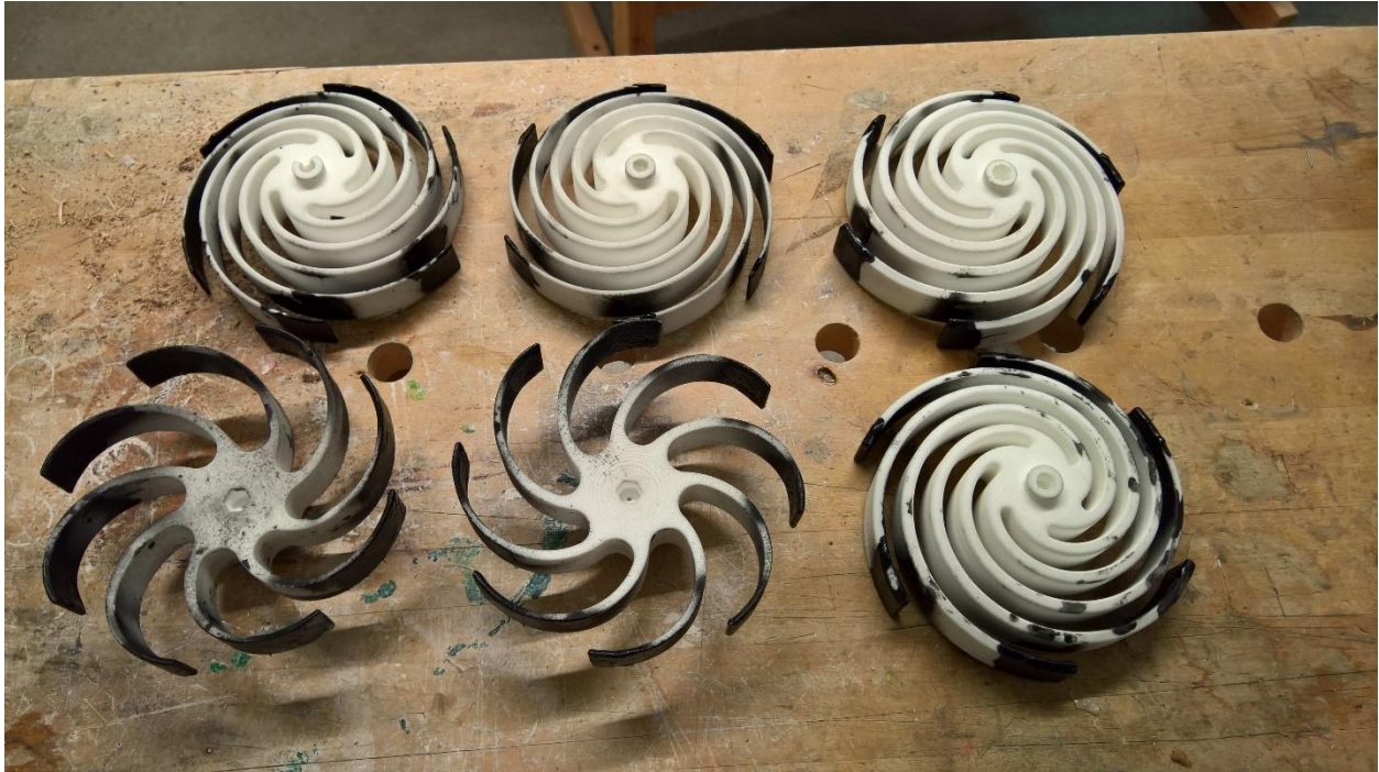
Figure 43 all wheel designs coated with liquid rubber
