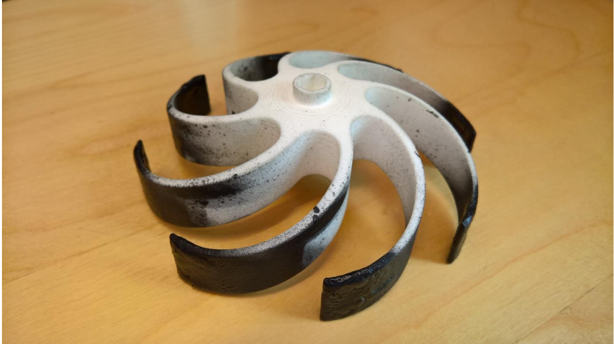
Figure 42 wheel design 1 coated with liquid rubber
