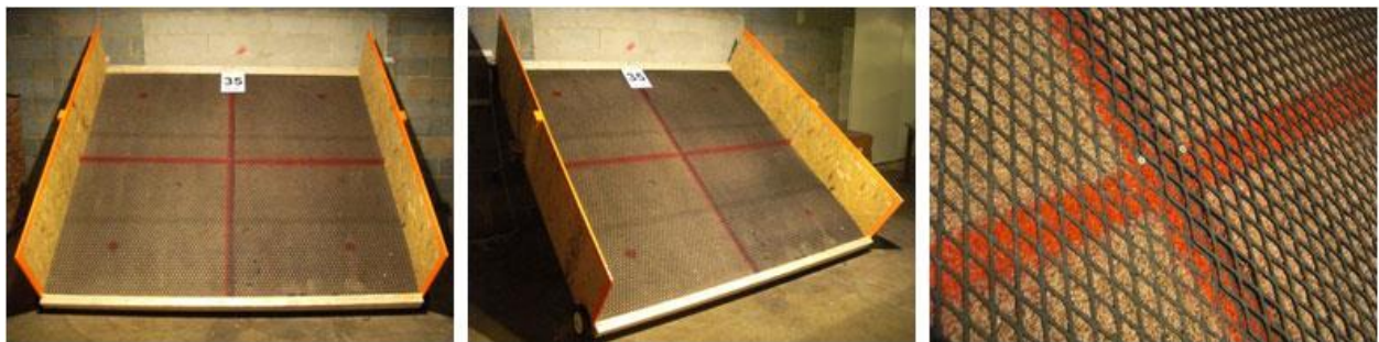
Figure 45 ASTM test standard E2803-11 Mobility: obstacle inclined plane (0° - 90°)
