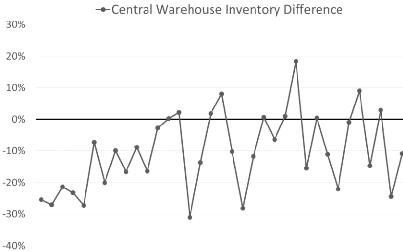
Figure 21 – The Relative Difference of BM Central Warehouse Inventory compared to Single-Echelon, Sorted by Increasing Fraction of Upstream Demand. Only Items Where Both Models Reach TSL for Upstream Demand are Included.
