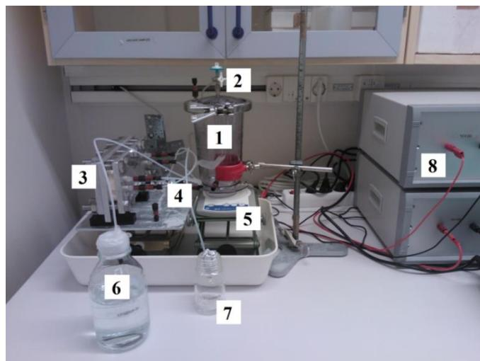
**Figure 3.8.** Ultrafiltration setup with 1) reservoir with stirring magnet, 2) air valve, 3) Tangential Flow Filter (TFF) cassette with Omega TM Membrane, 4) sterile Tygon tubing “PharMed-BPT”, 5) stirring plate, 6) permeate bottle, 7) retentate bottle and 8) power supply connected to a small membrane pump (membrane pump positioned behind the equipment)
