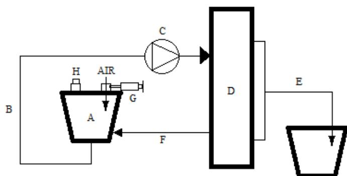
**Figure 3.9.** Ultrafiltration mode. A) Reservoir, B) Inlet line, C) Pump, D) Filter (300 kDa), E) Permeate line, directed to a permeate bottle, F) Outlet/Retentate line, connected to bottom inlet port, G) Lid inlet port connected to a syringe and H) Plugged lid inlet port
