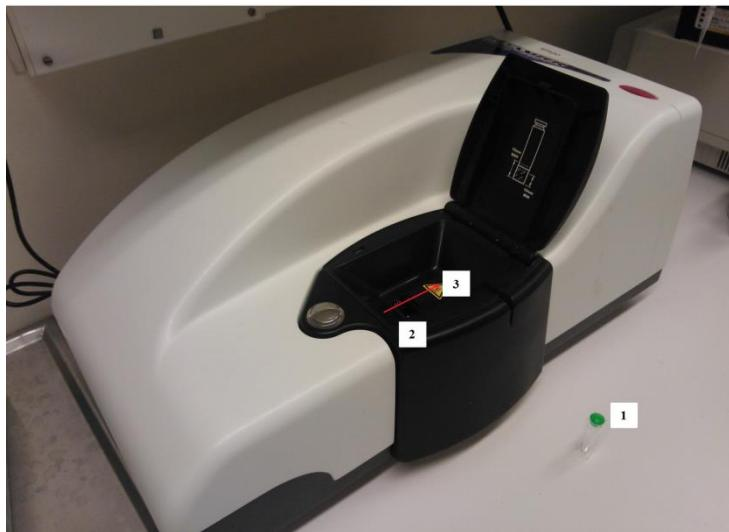
**Figure 3.6.** DLS equipment (Malvern Instruments, Zetasizer Nano-ZS). **1)** UV-cuvette micro **2)** Cuvette position **3)** Laser beam direction
