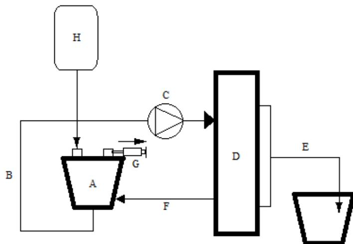
**Figure 3.10.** Diafiltration mode. **A)** Reservoir, **B)** Inlet line, **C)** Pump, **D)** Filter (100 kDa), **E)** Permeate line, directed to a permeate bottle, **F)** Outlet/Retentate line, connected to bottom inlet port, **G)** Lid inlet port connected to a syringe, used to create vacuum and **H)** MQ water tank connected to lid inlet port
