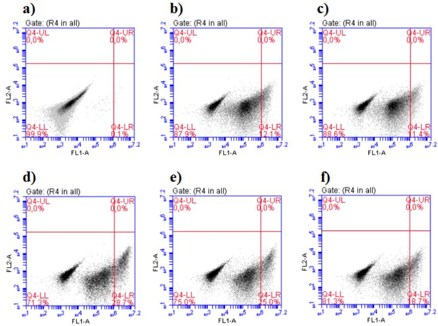
**Figure IX.V.** FL-plots for Raw264.7 cells (Experiment 2) after incubation **a)** without NPs and without primary antibody, **b)** without NPs, but with primary antibody, **c)** with bare NPs, **d)** with 100 mol% PEG6-9 coated NPs, **e)** with 100 mol% PEG21 coated NPs and **f)** with 100 mol% PEG44 coated NPs. Primary antibody was included in **b-f**.
