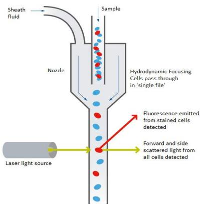
**Figure 3.18.** Principle of flow cytometry. The arrow marking detection of fluorescence points into the plane of the paper, orthogonal to the laser beam [43].
