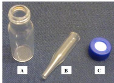
**Figure 3.5.** A) Vial, with accompanying B) 200 μL insert and C) lid
