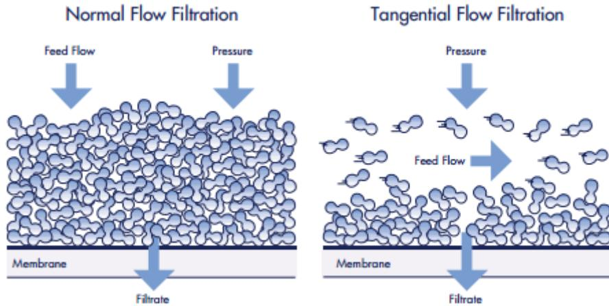
**Figure 3.7.** Two operational modes that can be used for filtration; NFF (left) and TFF (right). (Image reproduced from [23])
