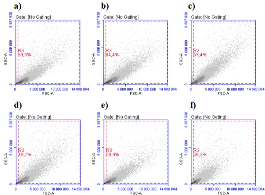
**Figure IX.I.** Scatter plots for Raw264.7 cells (Experiment 1) after incubation **a**) without NPs and without primary antibody, **b**) without NPs, but with primary antibody, **c**) with bare NPs, **d**) with 100 mol% PEG6-9 coated NPs, **e**) with 100 mol% PEG21 coated NPs and **f**) with 100 mol% PEG44 coated NPs. Primary antibody was included in **b-f**.
