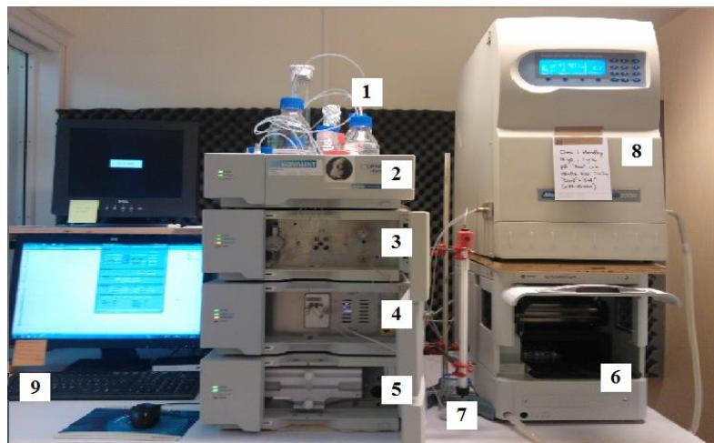
**Figure 3.4.** GPC equipment (YL9100 HPLC System). **1)** GPC running buffer, 50 mM  $(\text{NH}_4)_2\text{CO}_3$  pH 7.4 **2)** Vacuum degasser **3)** Quaternary pump **4)** PDA detector UV lamp **5)** Column compartment **6)** Autosampler **7)** Column (Superose™ Increase 10/300 GL) **8)** Evaporative Light Scattering Detector (ELSD) **9)** Computer with software
