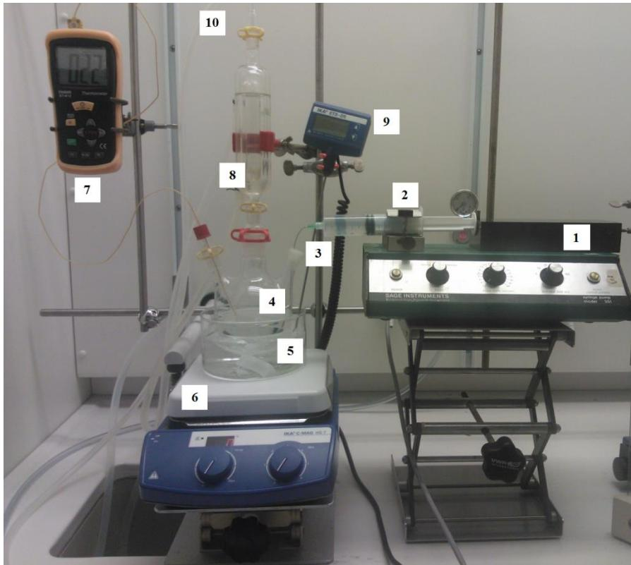
**Figure 3.2.** Coating equipment including **1)** syringe pump, **2)** 50 ml syringe, containing coating precursor, **3)** septum for sampling and coating injection, **4)** three-necked 500 ml reaction flask (round bottom), **5)** oil bath, **6)** hotplate stirrer, **7)** thermometer ( $T_{in}$ ), **8)** condenser, **9)** temperature sensor ( $T_{set}$ ) and **10)** line for  $N_2$ /vacuum.
