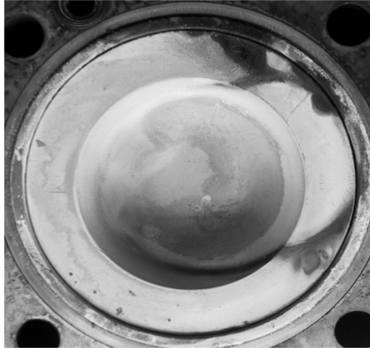
Figure 12 Picture of cylinder top after 1400 hours of operation.
