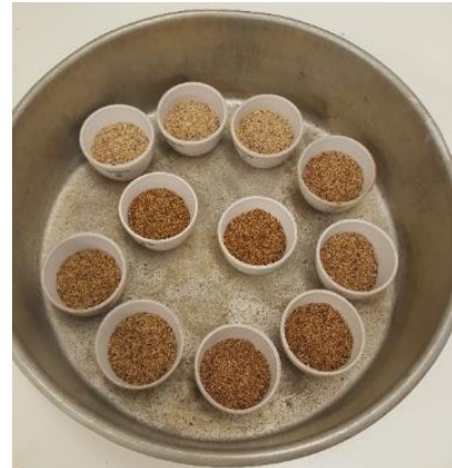
Figure 9. Samples ready to be burned in 550 °C overnight to then measured the ash content.
