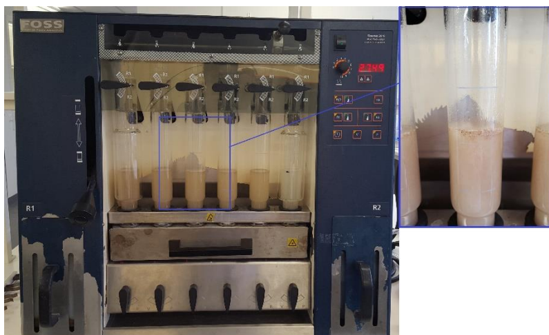
Figure 11. Tecator Fibertec 2010 Heat Extractor containing six crucibles that are placed under the boilers. At the bottom of the heat extractor the vacuum valve/air valve can be seen.
