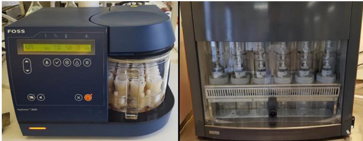
Figure 10. Hydrotec 8000 can be seen to the left (hydrolysis) and Soxtec Avanti 2050 Auto System can be seen to the right (end extraction).
