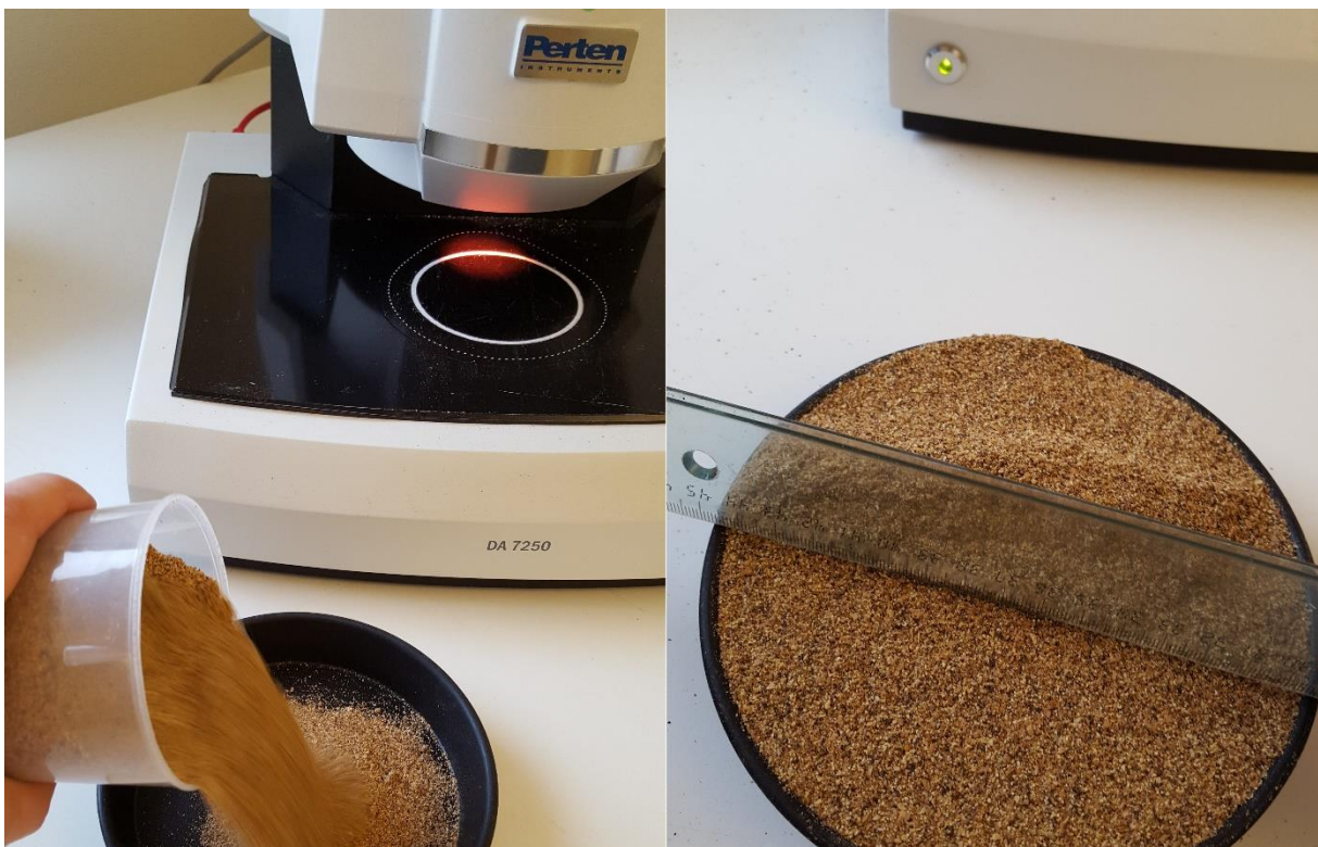
Figure 6. The samples were added to a plastic cup and by using a ruler a flat surface was obtained.
