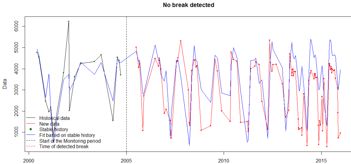
Figure 17. An example of pixel analysis from 2000 to 2015 (no break detected), where the black continuous line represents the historical data, the red continuous line represents the new data, the blue continuous line represents the prediction of the model. The vertical black dotted line represents the start of the monitoring period. In this case, the new data (red line) almost coincides with the predicted data (blue line)
