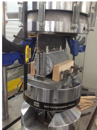
Figure 3.4: Test setup for testing the tensile strength of a cylinder specimen
