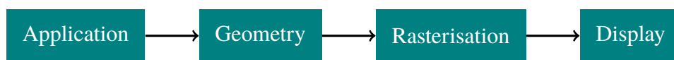
Figure 1.3: A very basic outline of the rendering pipeline. Application is where the 3D world resides and the Display is what the end user sees. All stages are explained in more detail below. Source: [14].
