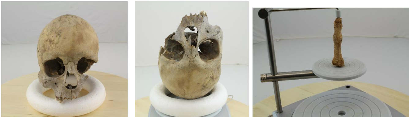
Figure 14. Left image: the cranium on the donut- shape styrofoam that hold it stable on the wooden rotating platform. Middle image: the cranium was raised by placing the cranium already placed on the styrofoam on the Autodrive platform. Right image: the metatarsal bone was held in place with the Part Gripper set on the Autodrive platform.
