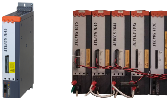
Figure 2.5 The ACOPOS 1045 Drive (left) [B&R Automation, 2015] and the ACOPOS setup used to control the FlexPicker robot (right).
