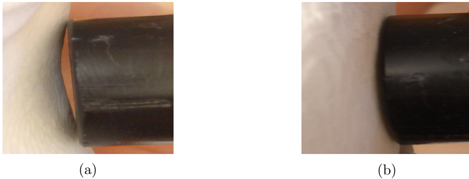
Figure 23: a) The detector placed on a curved surface where in between filled with ambient air. b) The detector is firmly attached on the model surface.
