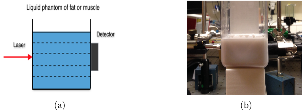
Figure 16: a) A drawn set-up on how to do the GASMAS measurement on the liquid phantom of fat and muscle: the liquid is in a transparent plastic bottle where the fibre and the detector are attaching the surface of the bottle. b) The set-up in the lab that is identical to the drawn set-up.
