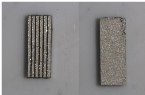
Figure 24. Back and front of a kerfed piezoelectric element.
