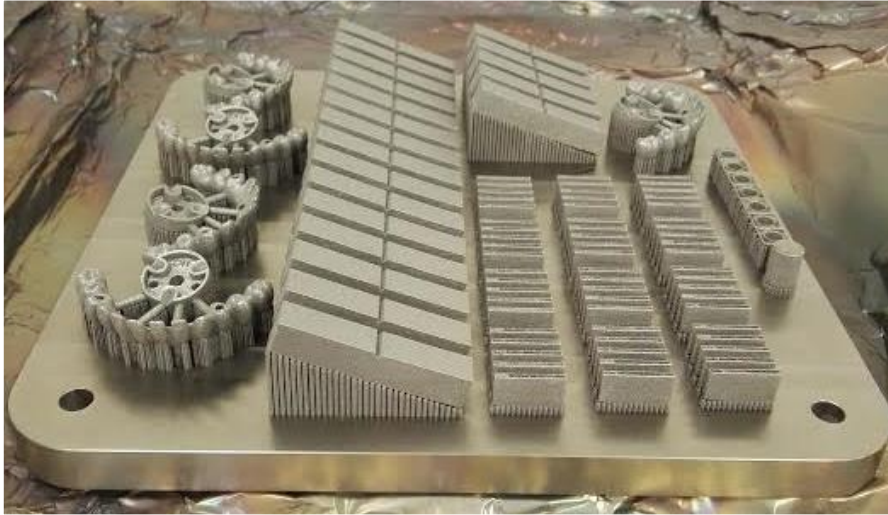
Figure 3.3 Printed build plate measuring 250 mm x 250 mm, showing five bridge structures with hubs, 20 Charpy samples, and 60 small plates as well as two artifacts to the far right of the picture.
