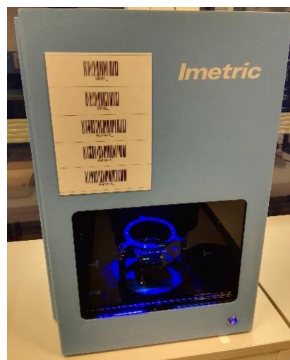
Figure 2.3 Imetric 3D scanner used in the process.
