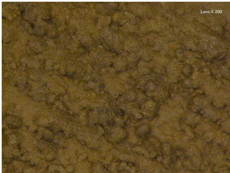
Figure 4.6 PEO coated surface at x200 magnification.
