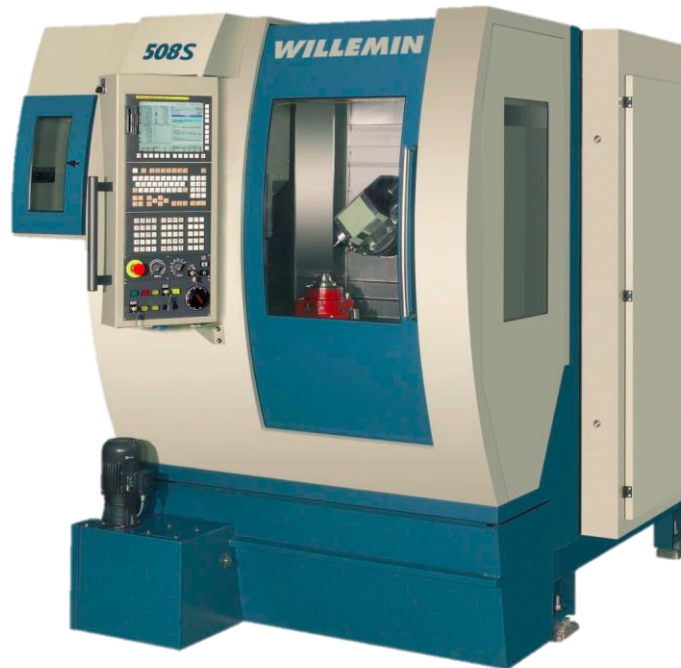
Figure 2.6 Milling machine used to mill implant interfaces.
