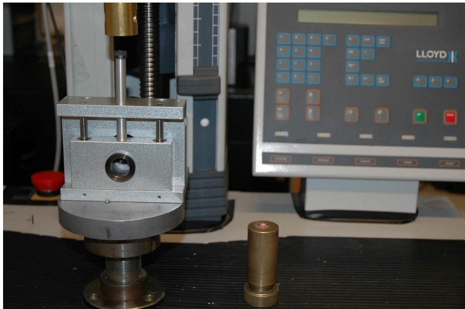
Figure 3.5 Bond strength testing setup.
