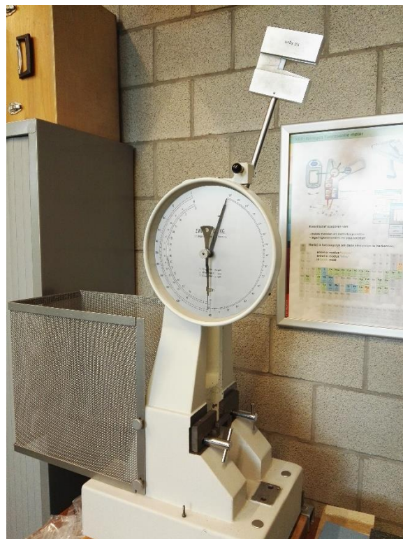
Figure 3.6 Charpy impact setup with 14.7 Nm pendulum.
