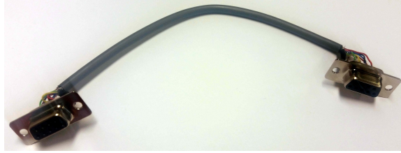
Figure 35: The wire used to connect the slave module with each other and also provide power supply and serial communication with the master.
