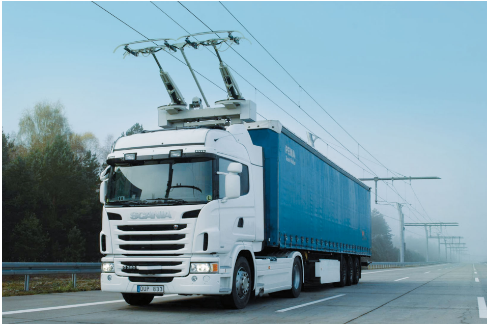
Figure 3: Siemens concept eHighway with overhead lines. [5]
