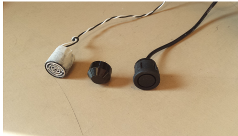
Figure 22: The three different transducers that were tested in the project all of piezoelectric type. From left to right: Unsealed transducer from lab, sealed transducer from lab and Biltema transducer
