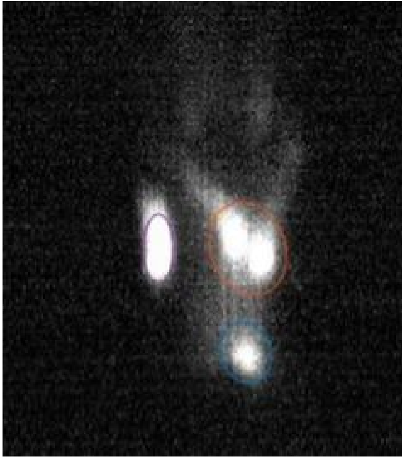
Figure 5.13: Multiple features after calculation. As can be seen only three points can be chosen with good results, while the last will be discarded due to overlap
