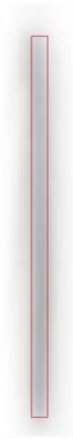
Figure 4.16: Images when slit is used together with calculated size by the MATLAB algorithm. Height of this slit became 28.7 mm (575 Pixels) and the width became 1.3 mm (26 Pixels).
