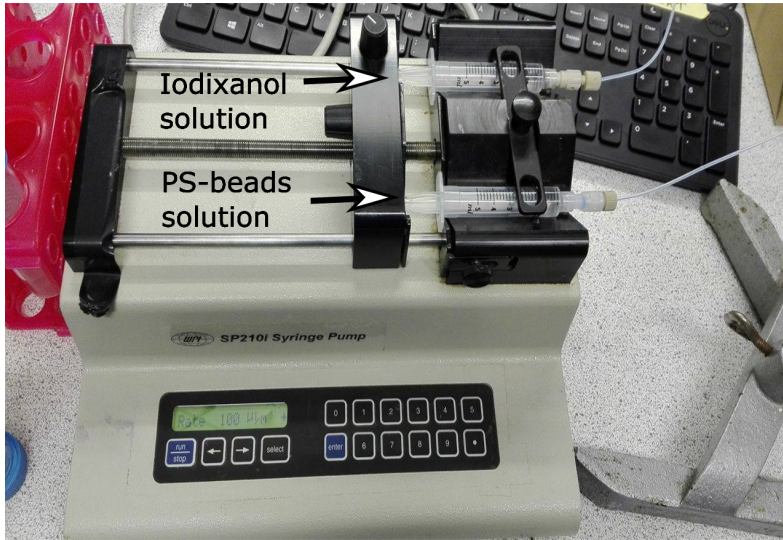
Figure 4.8: The syringe pump set up showing the iodixanol- and PS-bead solutions during aim 3. The flow rate was set to 100 \mu\text{l}/\text{min} .
