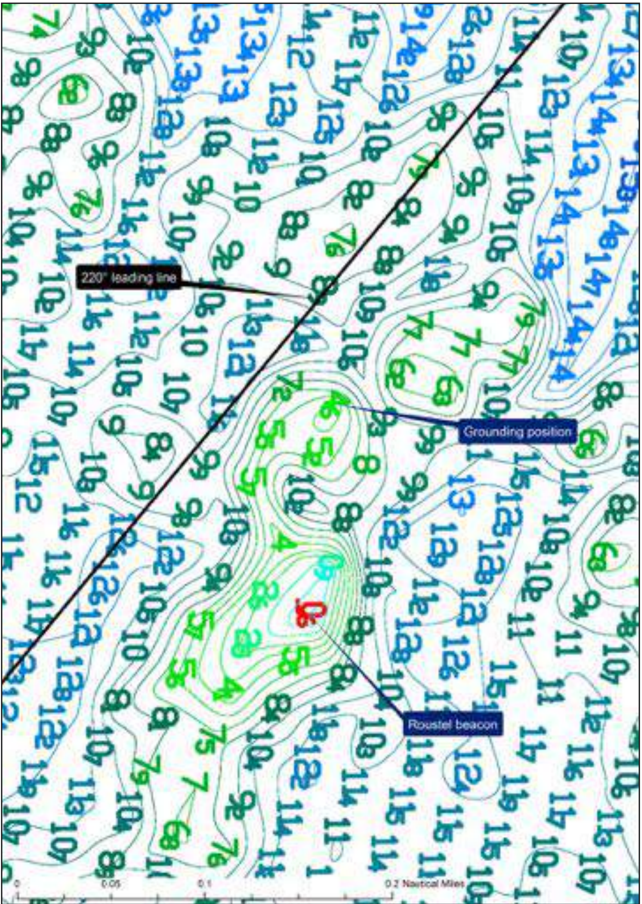
Figure 19: Extract of data from multi-beam survey conducted in March 2014 showing 4.6m sounding in grounding position (orientated north up)
