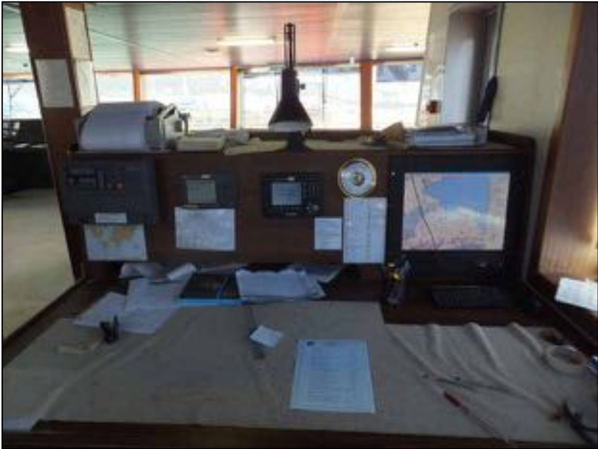
Figure 7: ECDIS planning terminal
