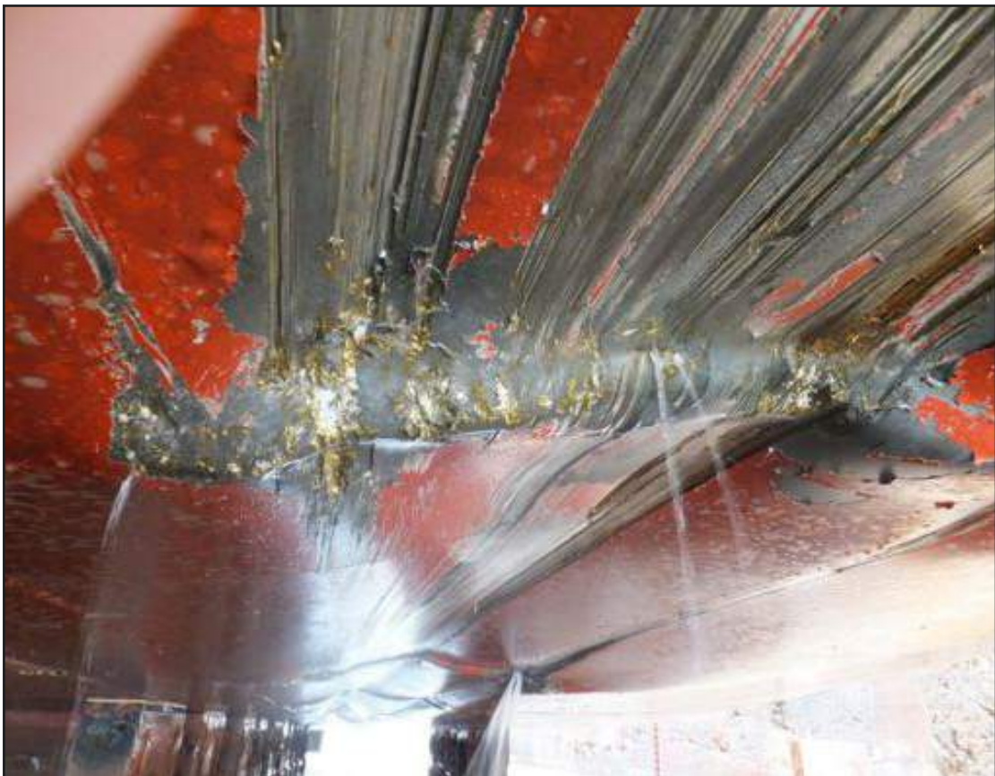
Figure 10: Detail of hull fracture damage
