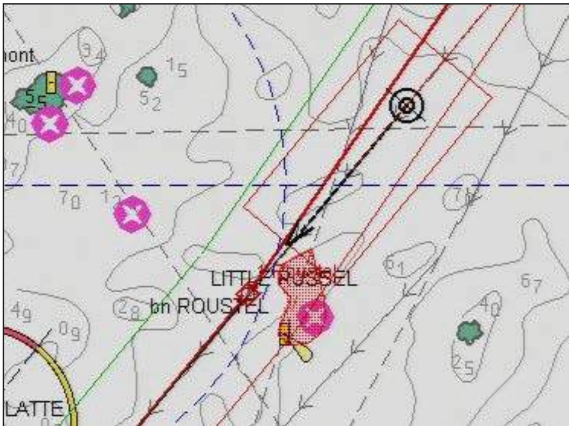
Figure 30: Reconstructed ECDIS display showing safety frame crossing 6.3m LDL
