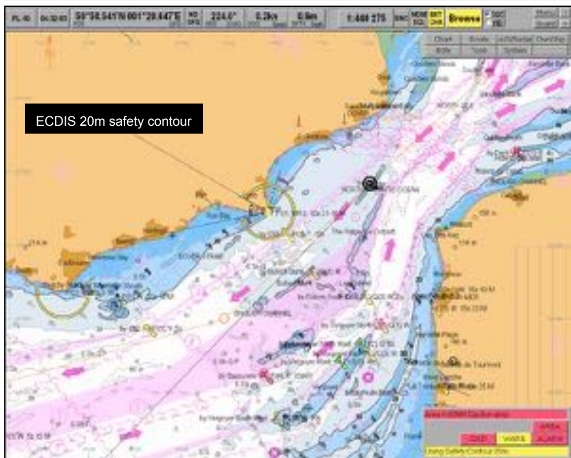
Figure 13: ECDIS display comparison of 30m and 20m safety contours
