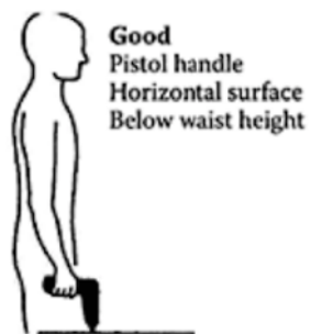
Figure 5.3: The figure shows a good position of the hand, wrist and arm. The pistol handle on horizontal surface are used in the created prototype (Helander Martin, 2006)
