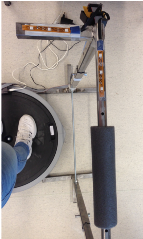
Figure 4.16: The prototype after the flexi-led-light was moved. This prototype was used during the second test with a stroke-survivor.
