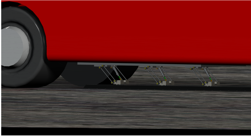
Figure 35: Finished design with ERS seen as a rendered image mounted underneath a bus
