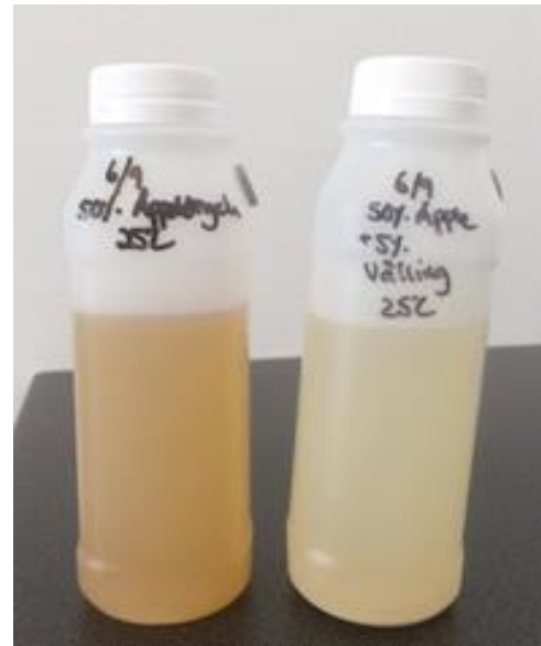
Figure 1. A plastic bottle with 50% apple juice to the left and a bottle with ProViva apple drink to the right. The bottle to the right has a changed structure and can't stand up straight anymore due to gas formation.
