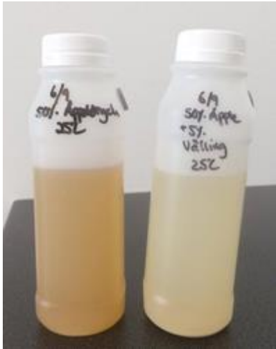
Figure 5. A plastic bottle sample with 50% apple juice to the left and bottle with 50% apple juice and oat swell to the right. The bottle to the right has a changed structure and can't stand up straight anymore due to gas formation.
