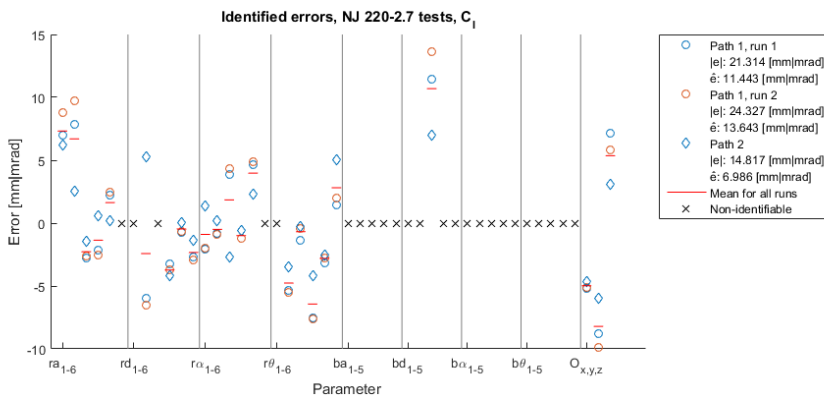
Figure 5.12 Identified errors using C_\ell for different robot paths, of which two are identical but captured during two different experiments.
