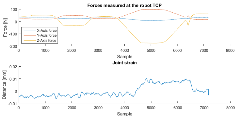
Figure 5.9 Ball-bar joint backlash when changing ball-bar force direction.
