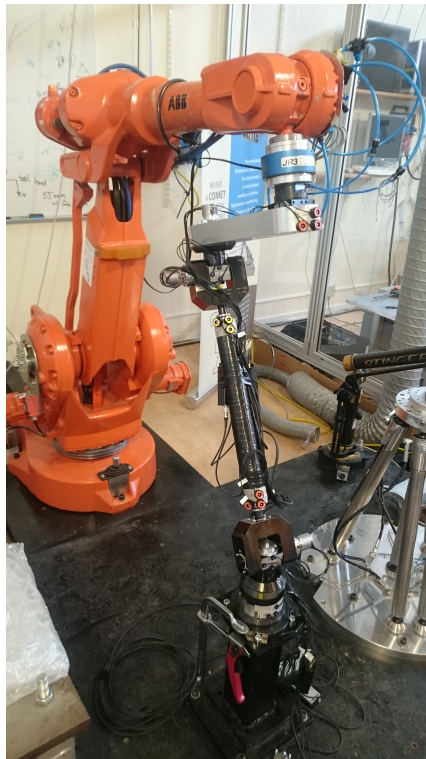
Figure 5.6 The ABB IRB 2400 robot with force-torque sensor, offset plate and the double ball-bar mounted.
