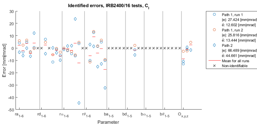
Figure 5.15 Identified errors using C_\ell for different robot paths, of which two are identical but run with different speeds.
