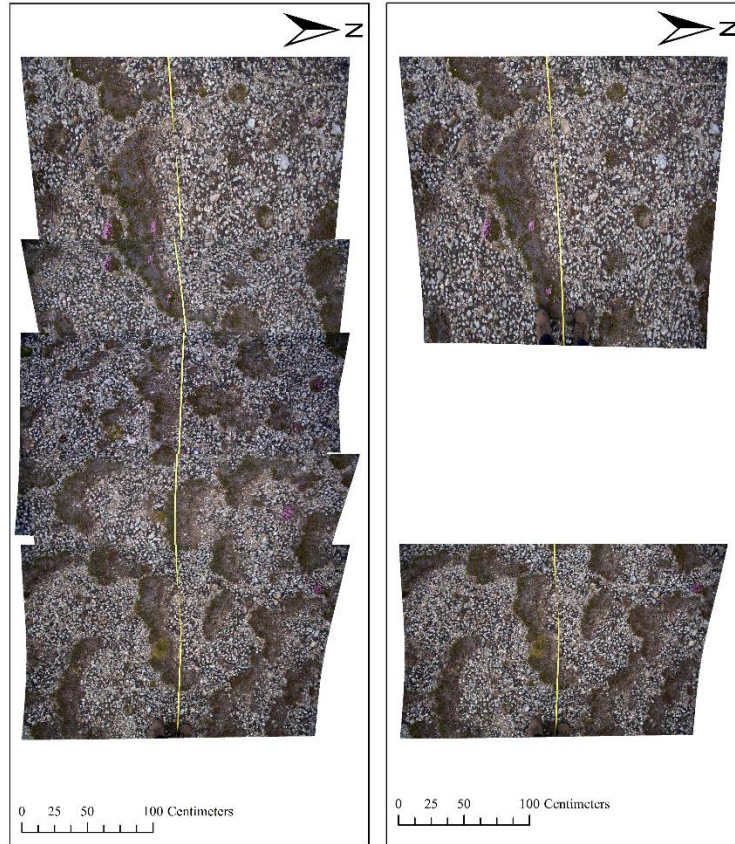
Figure 10. An example of the distortion using method 2. Five images in a column (left) and image 1 and 5 (right).
