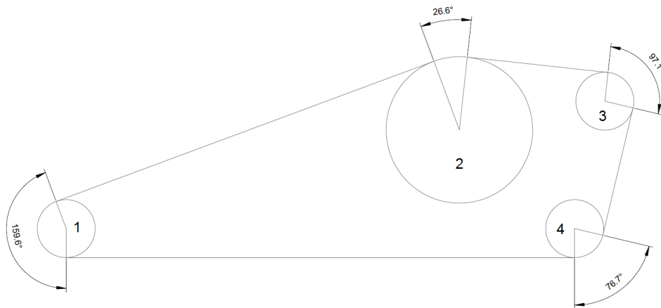
Figure 8.10. Pulley and belt set-up with wrap angles.
