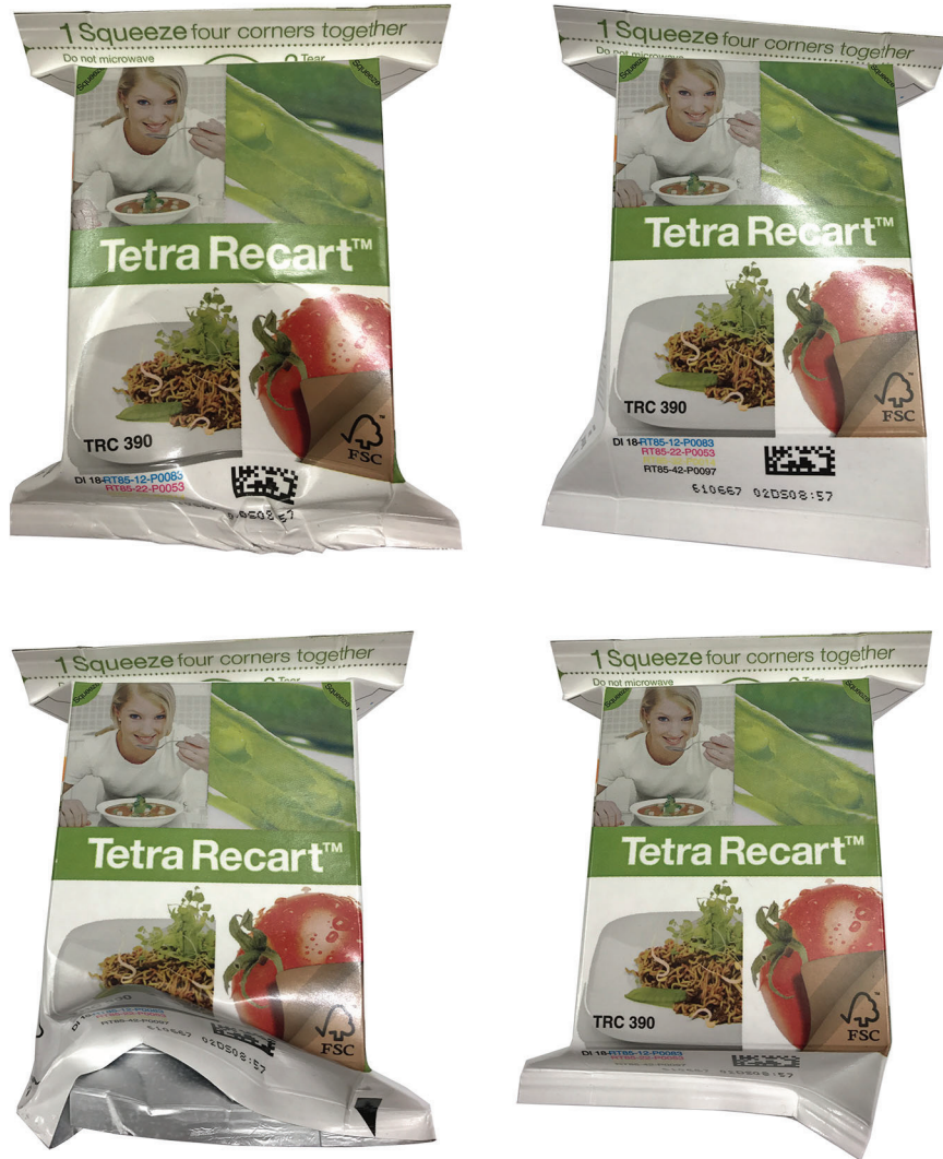
Figure 6.1. Examples of faulty packages.
