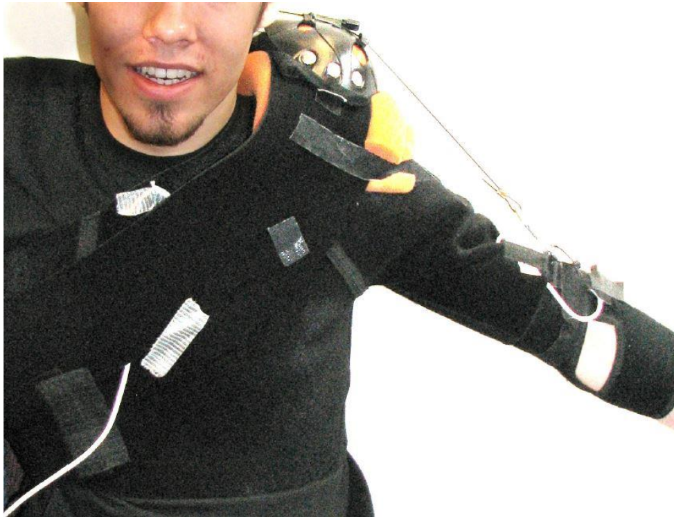
Figure B.1 Active Soft Orthotic System for Shoulder Rehabilitation [5]
