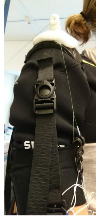
Figure 7.3 Left: T-shaped rail attached to extended backplate, right: strap from shoulder part to elbow brace
