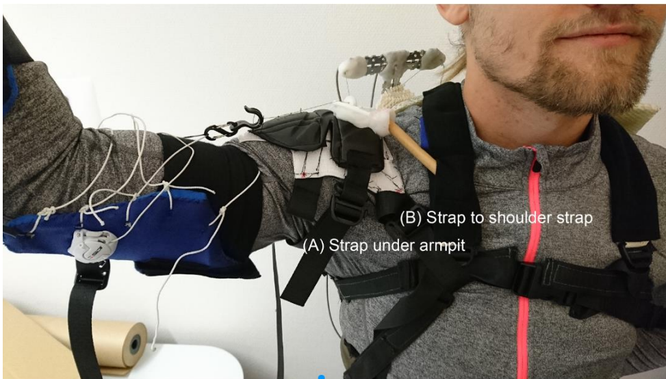
Figure 8.7 Clavicle aligned support as wooden rod with straps
