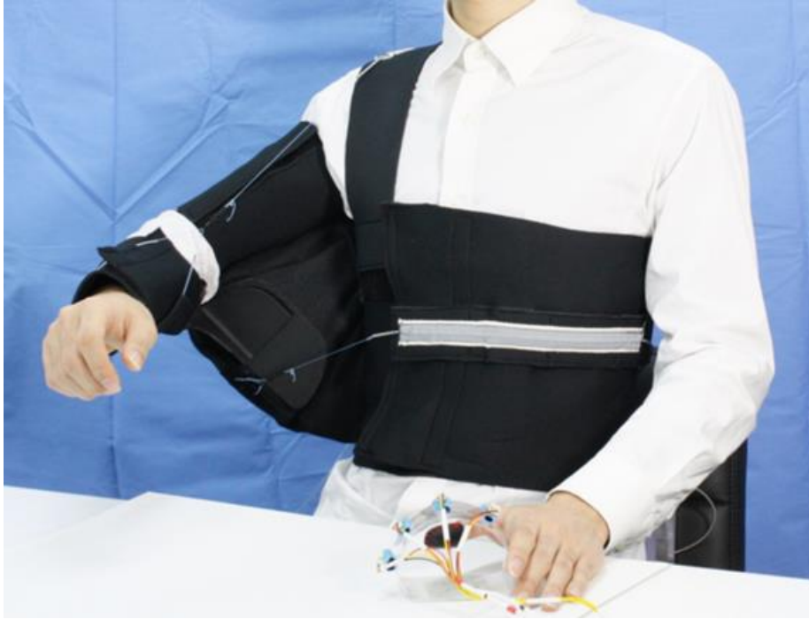
Figure B.4 Meal Assistive Exoskeleton made of Soft Materials for polymyositis patients [8]
