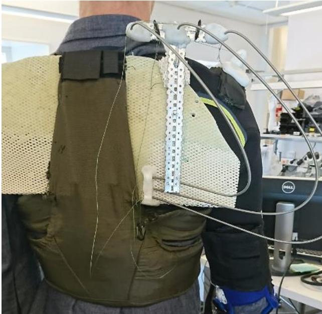
Figure 7.3 Left: T-shaped rail attached to extended backplate, right: strap from shoulder part to elbow brace
