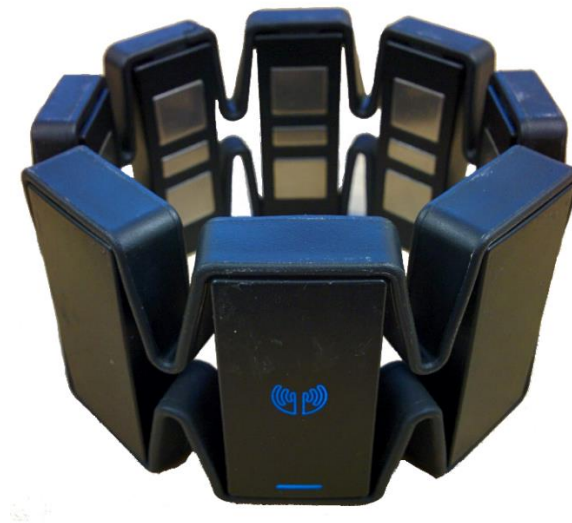
Figure 11: The Myo™ armband. The eight electrodes are connected via flexible sections that can be stiffened by attaching clips, making the armband able to snugly fit around the lower arm.
