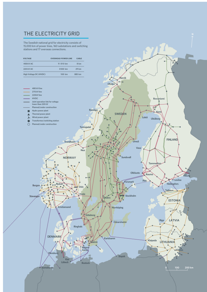
FIGURE 2.1: Map of the electricity grid in Sweden, from (Svenska Kraftnät, 2016b).
