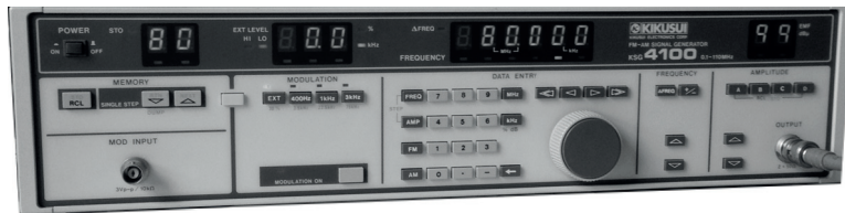
Figure 5.1: KSG4100 generating a 80 MHz signal
