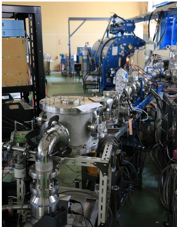
Figure 4.3: A picture of the Pelletron beamline with target chamber setup.
