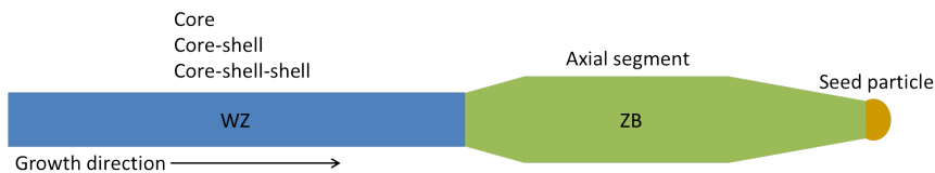
Figure 3.1: A schematic structural overview of the type of nanowire. The desired structure is the WZ InAs-GaSb(-InAs) core-shell(-shell) nanowire, and the axial segment of GaSb is a result of the shell growth.
