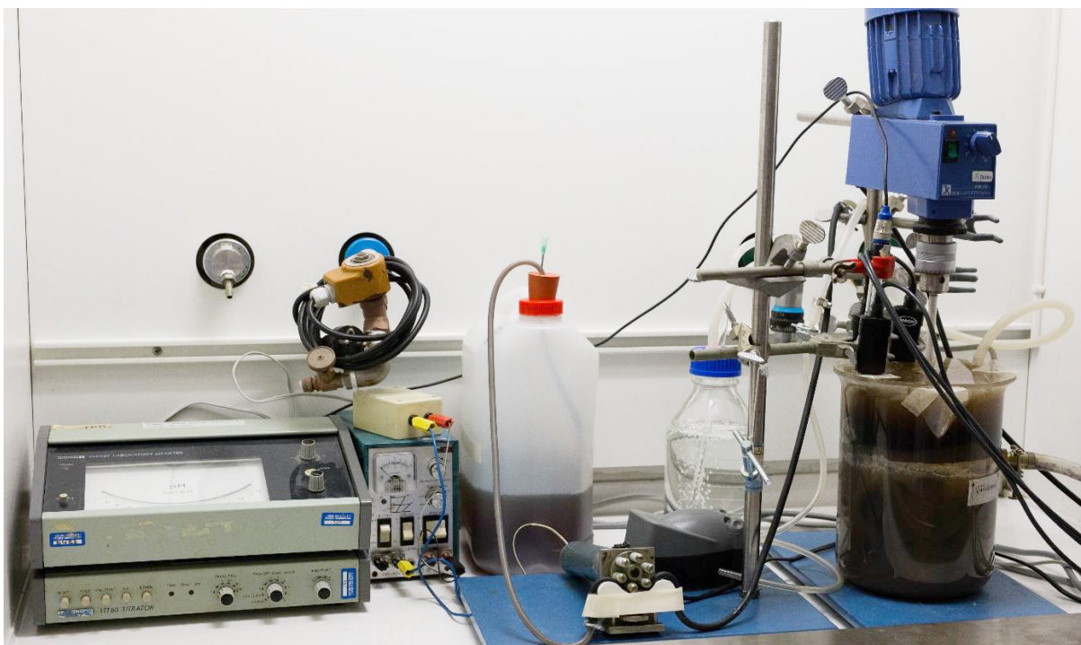
Figure 5.3. Process setup with pH-regulated influent. The effluent container is not shown in the picture.
