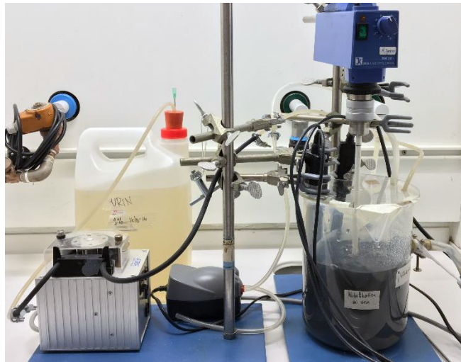
Figure 5.2. Process setup with fixed-flow influent feed. The effluent tube is placed on the right, the effluent container is not shown in the picture.
