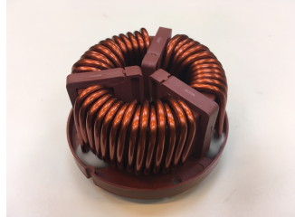
Figure 67: HVAC common mode filter.
