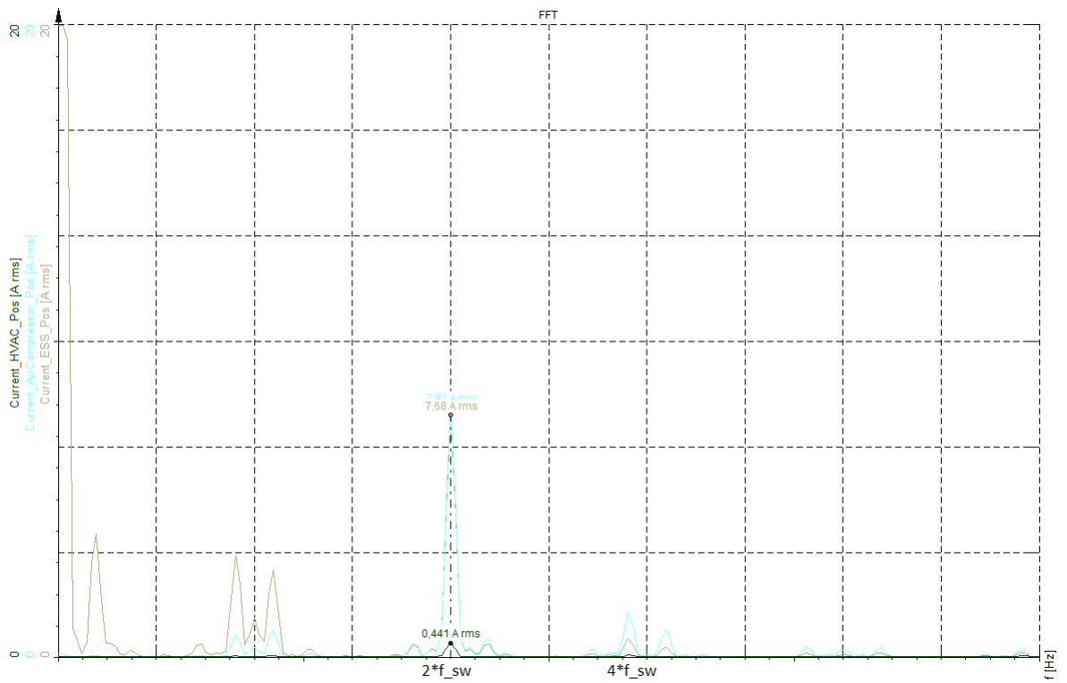
Figure 76: FFT of the subsystems current ripple with EMD and DCDC active. The speed of the EM is here around \frac{\omega_{basespeedEM}}{2} . Frequency and current plotted.
