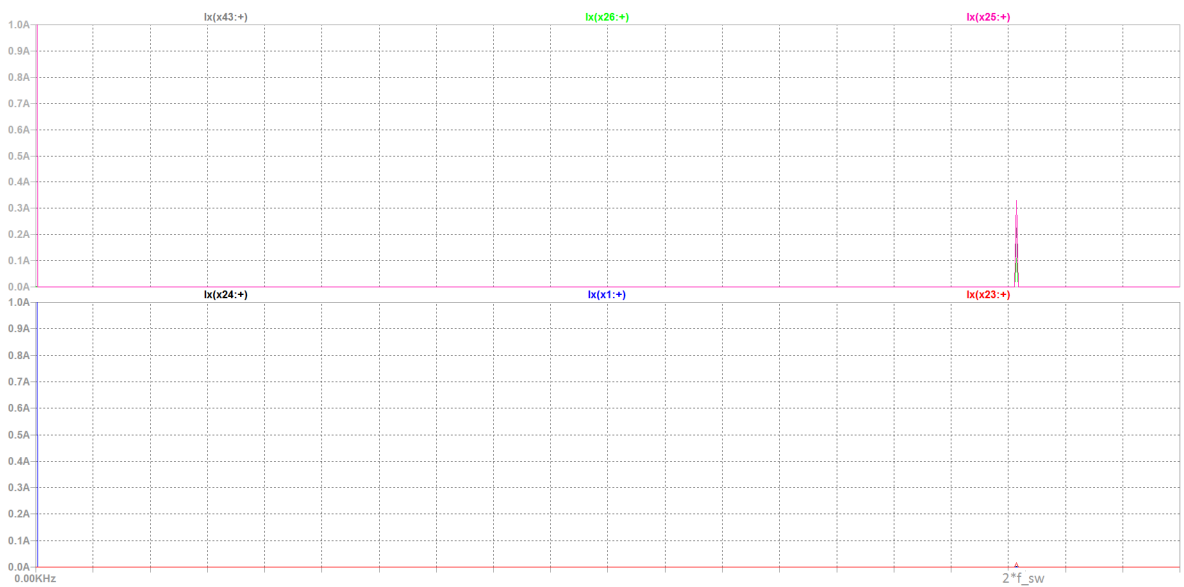
Figure 51: FFT of the subsystem currents when the DCDC was simulated. The light green represents the DC-voltage, the blue the ESS current, the red the air compressor current, the black the OnBc current, the pink the EMD current, the grey the HVAC current, and the dark green represents the DCDC current.
