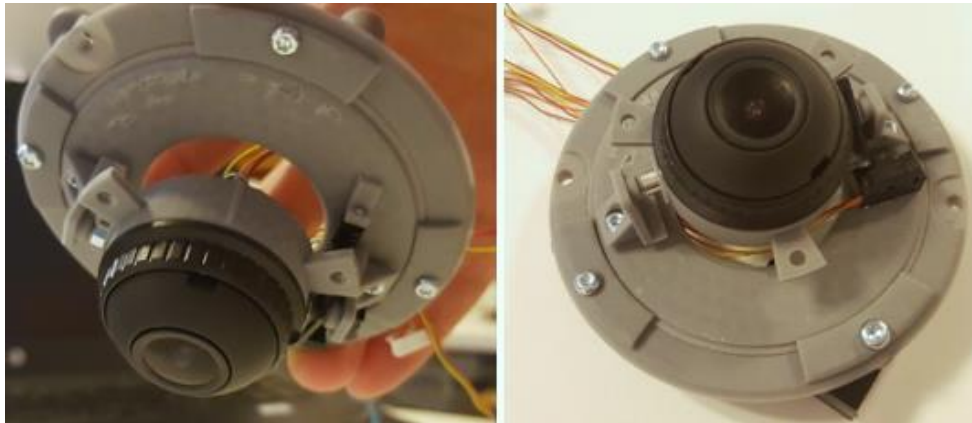
Figure 11.5: Prototype without rotate gear.
