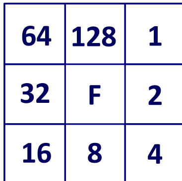
Figure 3. Encoding of neighboring cells used for the flow directions in the D8 algorithm with F indicating the focus cell.
