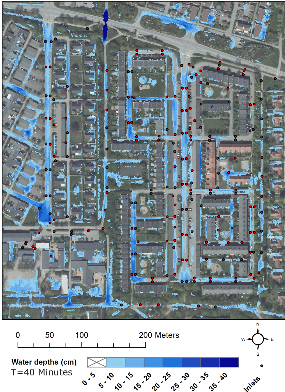
Figure 26. Water depths at T=40 minutes. 10 minutes has passed since the rainfall stopped and now the water is just flowing and infiltrating in permeable areas and into the storm sewer inlets. The settings are explained in Figure 23. GSD-Ortophoto, 0.5 m color © Lantmäteriet (2014).
