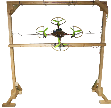
Fig 4.15: The quadrotor platform test rig.
