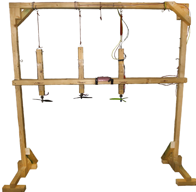
Fig 2.5: Motor and propeller test rig.
