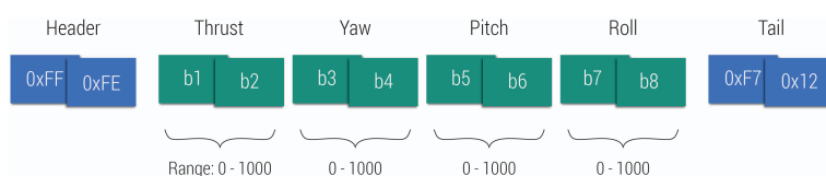
Fig 4.27: A flight control frame in the improved platform protocol.
