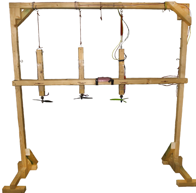
Fig 2.5: Motor and propeller test rig.
