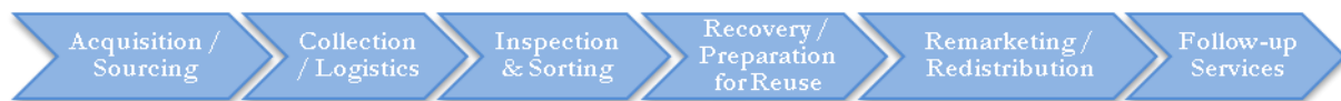
Figure 2-2. Range of activities potentially covered by organisations engaged in computer reuse illustrated as a chevron process
