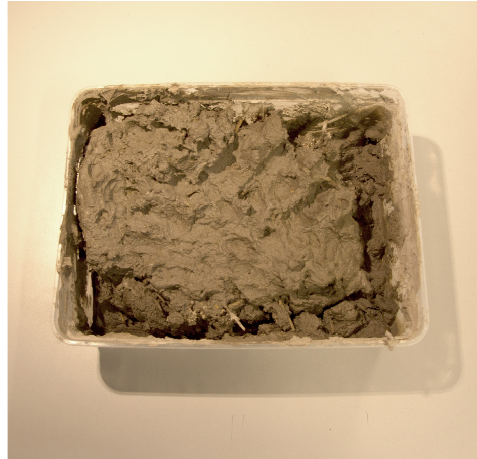
Brick mixture of 1/3 soil, 1/3 sand and 1/3 silt
