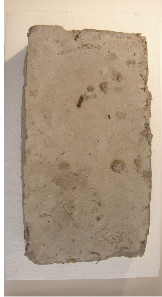
Brick with 1/3 soil, 1/3 sand and 1/3 silt
