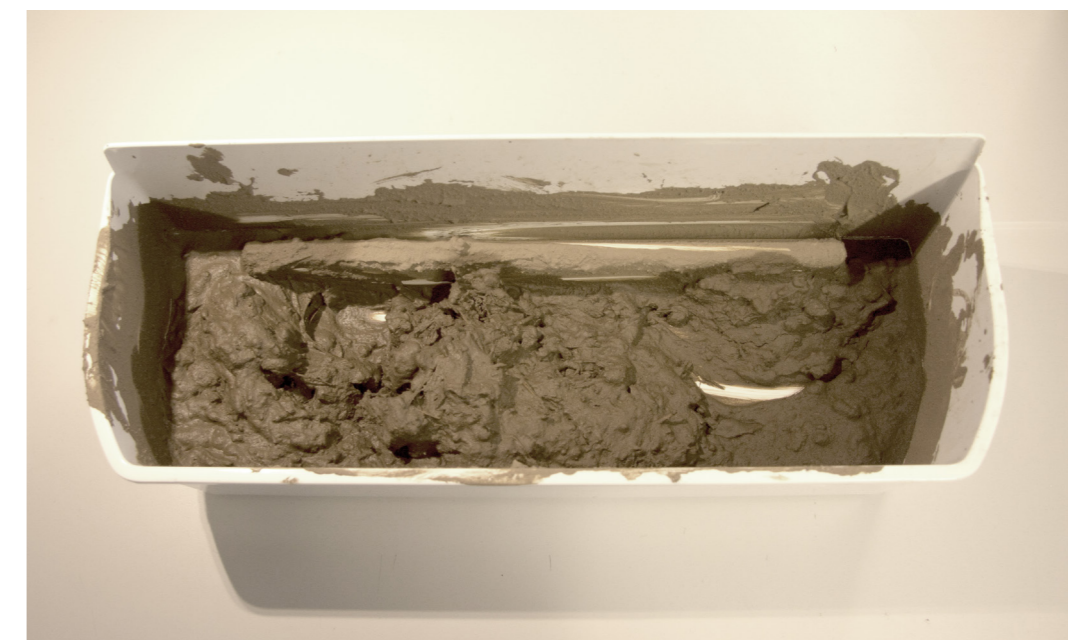
Brick mixture of majority sand
