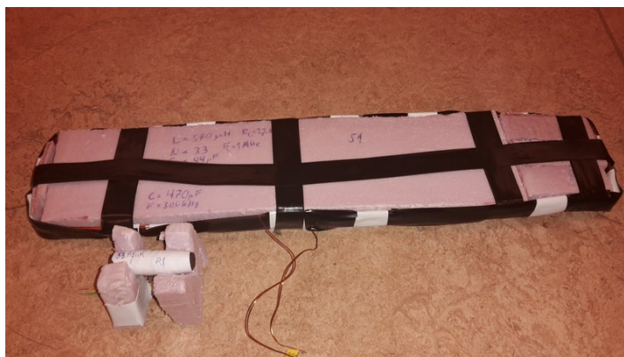
Figure 4.7: The transmitter (top one in picture) and receiver antenna, at an earlier resonance tuning. The dimensions and shape are the same as in the chosen 140 kHz setup. Only the number of windings and the tuning capacitance value differ.
