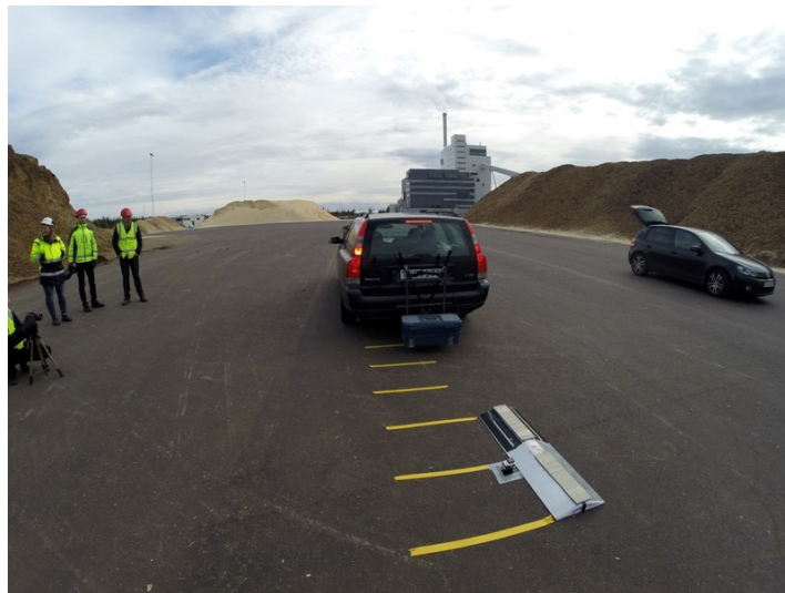
Figure 4.20: The rail mock-up at the Örtofta test location. A high speed camera can be seen rigged in the far left of the picture.
