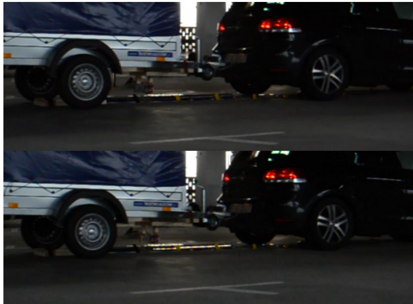
Figure 4.36: The detection and turning on of the first rail segment represented by the LED strip in front of the trailer tires.
