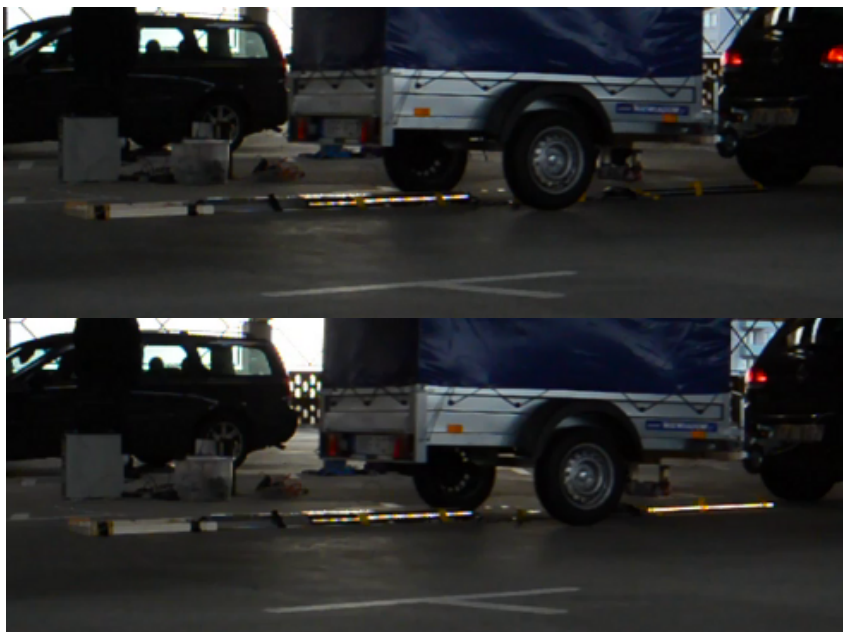
Figure 4.37: The detection and turning on of the second rail segment represented by the LED strip in front of the trailer tires.
