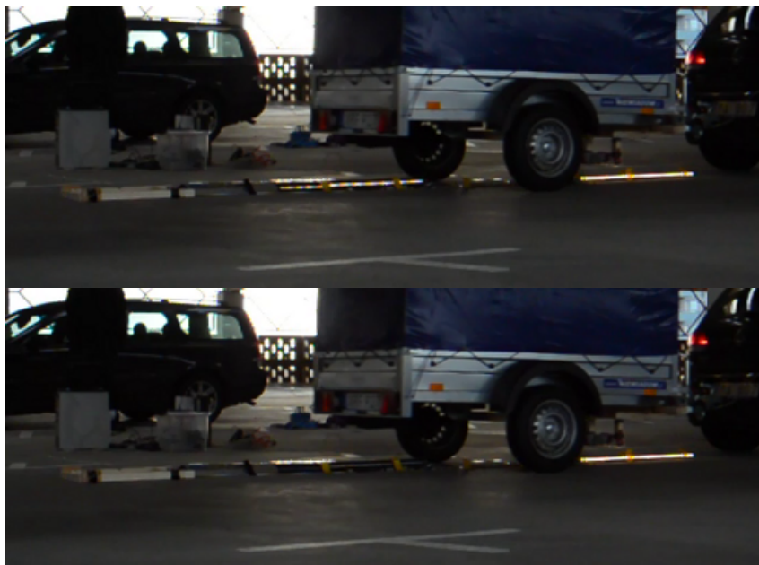
Figure 4.38: The timing of the first rail-computer (Arduino) turning off the first rail segment represented by the LED strip behind the trailer.
