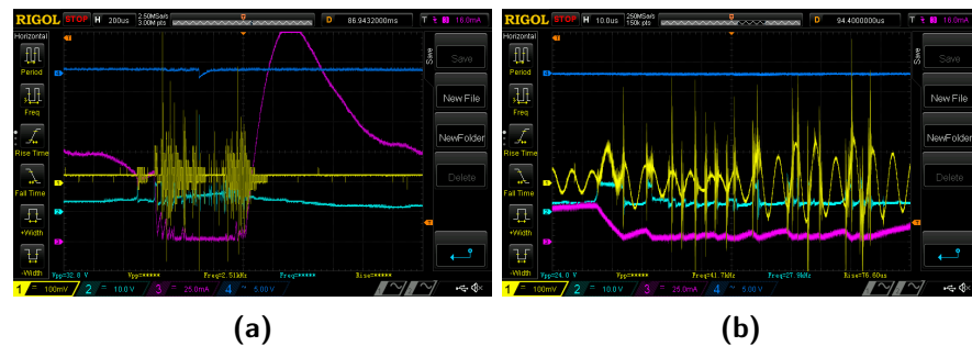
Figure 4.29: The ringings in the receiver antenna when the loop antenna was placed at a 90 degree angle with the rail and the current was 80 A in left picture and 40 A in right picture
