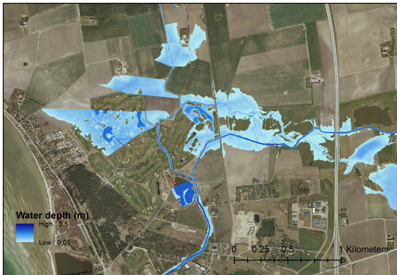
Figure 7.7: Inundation extent when the main channel is separated from the overbanks by adding levees to 1D cross section. Background image GSD-Ortofoto, 1m color ©Lantmäteriet.
