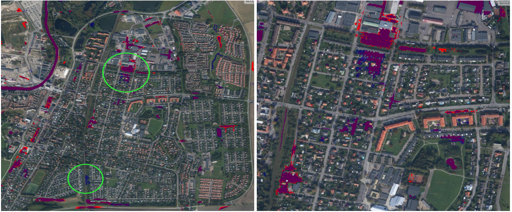
Figure 8.16: Areas with inundation depths larger than 0.2m, generated after 2 hours of simulation using 4m (blue) and 16m (red) computational mesh sizes respectively. Results are shown for the whole area (left) and for a smaller (zoomed in) part (right).
