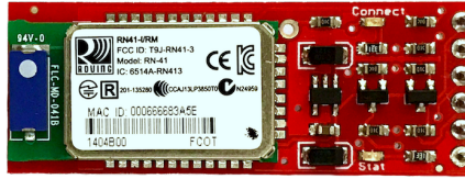
Figure 3.12: Bluetooth breakout board for Arduino
