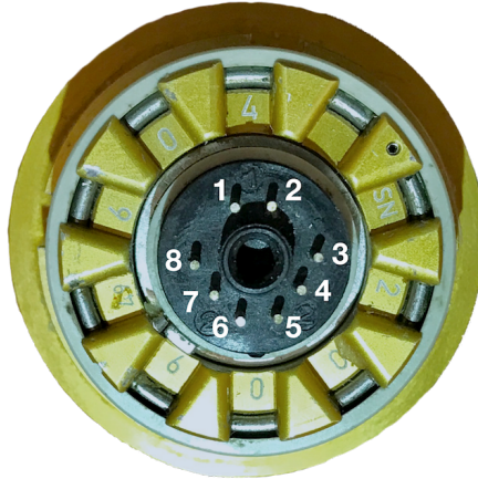
Figure 3.13: The pins of the Ottobock hand.
