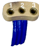
Figure 3.19: The pin connection of the EMG sensors (see appendix A.6).
