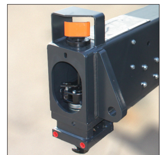
Twistlock and lifting eye.
