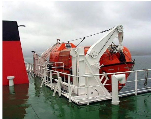
Figure 5 shows a lifeboat with its gravity launched davit system. Picture is taken from: (Nautic Expo, 2016a)
