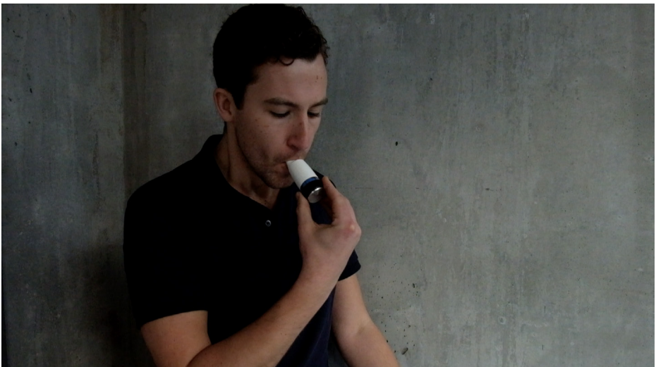
Figure 7.6.4 The light turns off when an inhalation is being made (the glass empties). Then the inhaler blinks for 10 seconds to remind the user to hold his breath.
