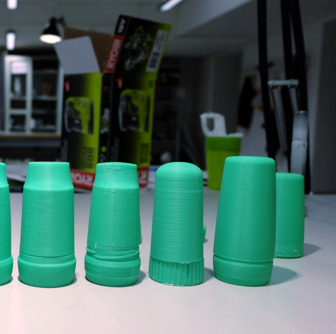
Figure 6.4.1. Prototypes were printed to understand what the inhaler would feel and look like.
