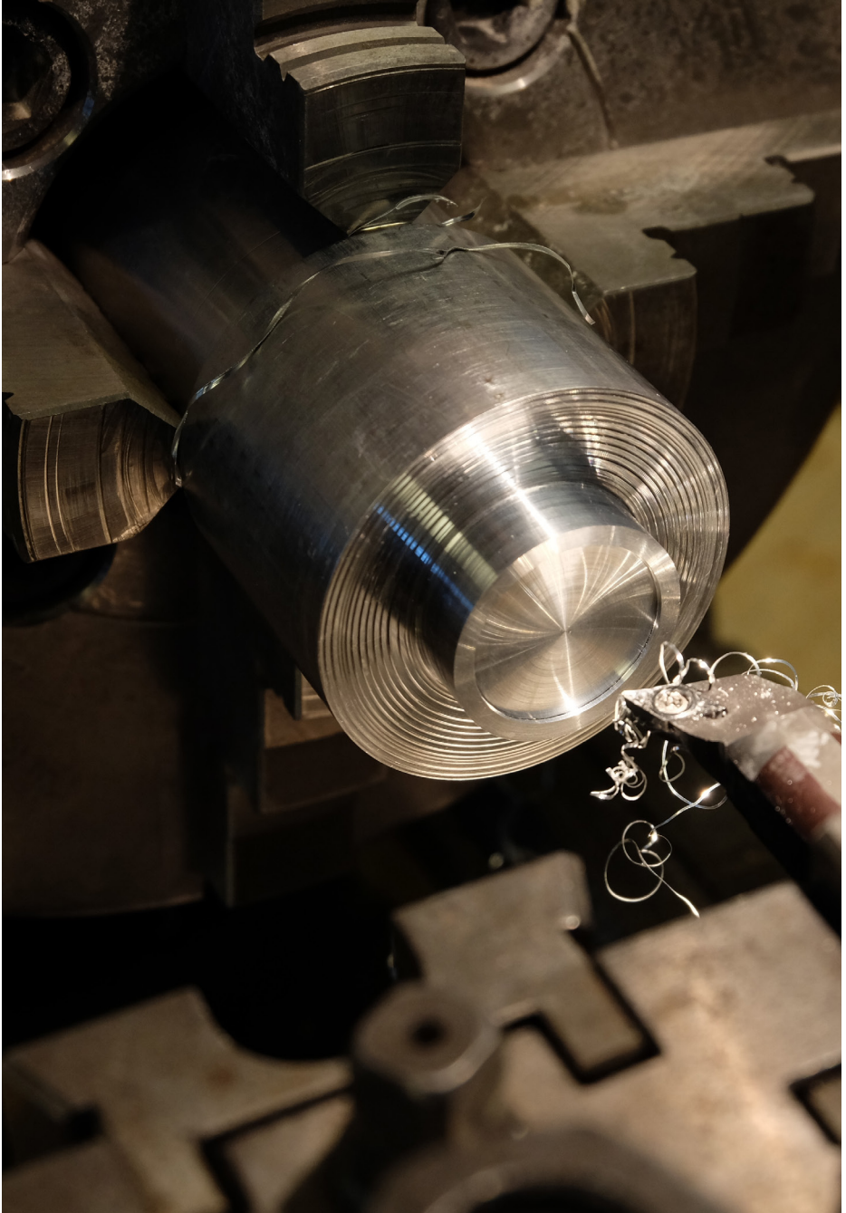
Figure 7.7.1 Prototyping the first aluminium casing.
