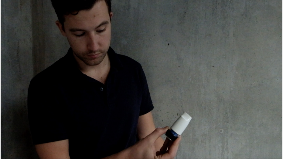
Figure 7.6.1 The lights are off when the inhaler isn't held upright. Visit https://youtu.be/PARRxuVbmjg for a video.
