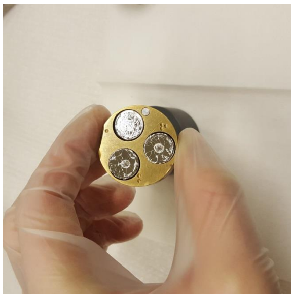
Figure 5.2. Sample holder for SEM, which can hold three individual samples. These can be inserted into the microscope at the same time. In this image the samples have been sputtered with Au/Pd layer.
