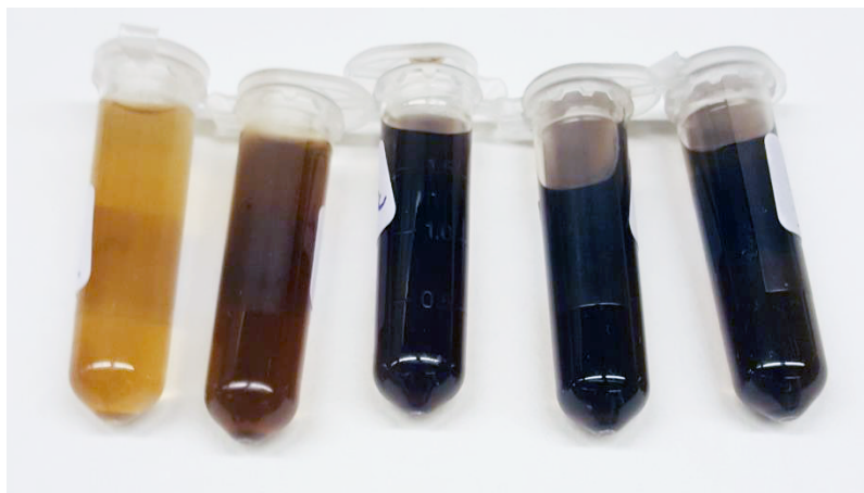
Figure 7.1. Acid hydrolysis time starts to the left with one hour and end with a reaction time of 5 hours to the left, with one hours increase between the cuvettes
