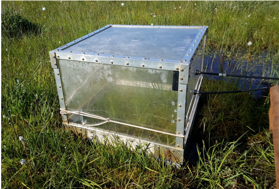
Figure 2: The 41l Plexiglas chamber sitting on top of the 30 x 30cm aluminum base. Inside is a small fan and to the right are the inlet and outlet lines which deliver the gas sample to the Gaset DX 40-30 FTIR spectrometer (image: Joel White).
