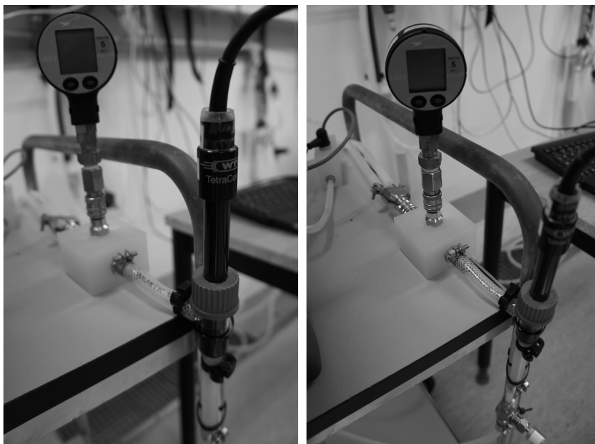
(a) WTW Cond 3110 conductivity sensor
