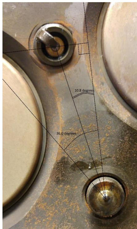
Figure 5 Spark location between fuel sprays.
