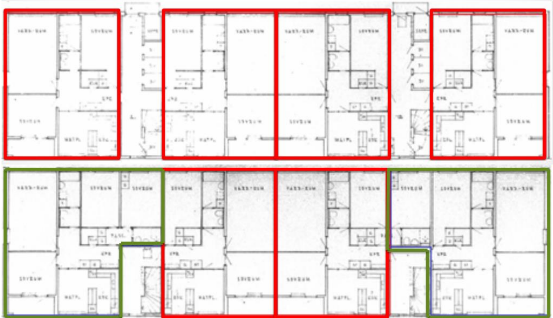
Figure 2.4 Floor plans, original drawings. Ground floor (upper) and first floor (lower). There are in total six two-bedroom apartments (red) and two three-bedroom apartments (green).
