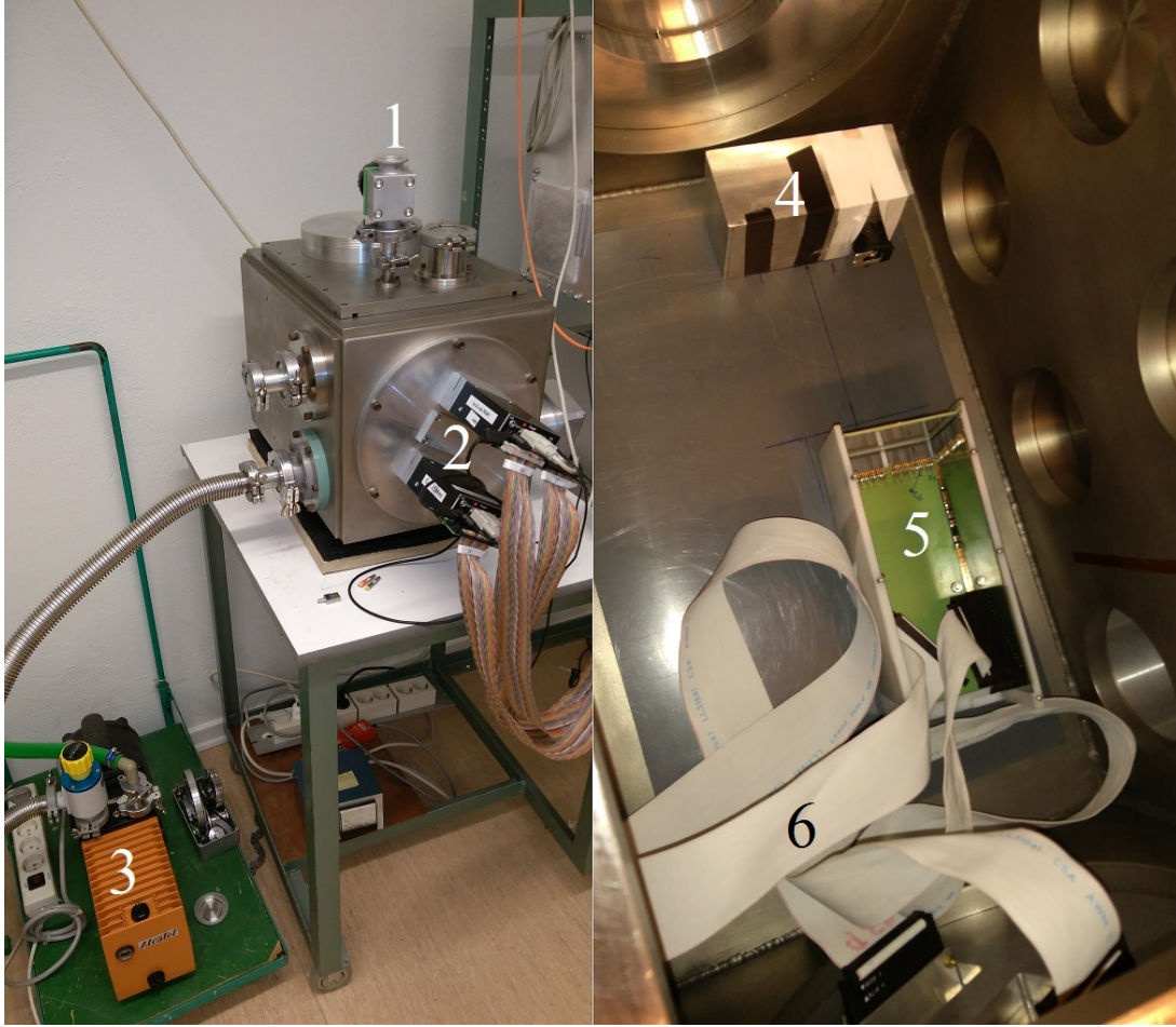
Figure 10: a) shows the outside of the vacuum chamber and b) shows the inside of the vacuum chamber. 1- air valve, 2- vacuum feedthrough and preamplifiers, 3- vacuum pump, 4- mounted source, 5- DSSSD and 6- flat ribbon cable.
